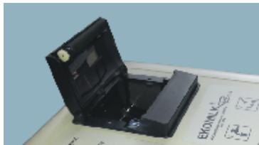
2.2. Open the cover and remove the used paper roll spool if one is in the paper roll compartment.
